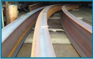
Bending Of Structural Steel
